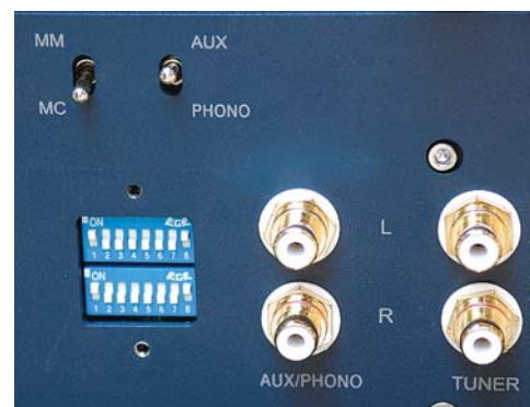
Perfect adjustable Lp. stage, MM/ MC (from 0,4 mV sensitivity)
